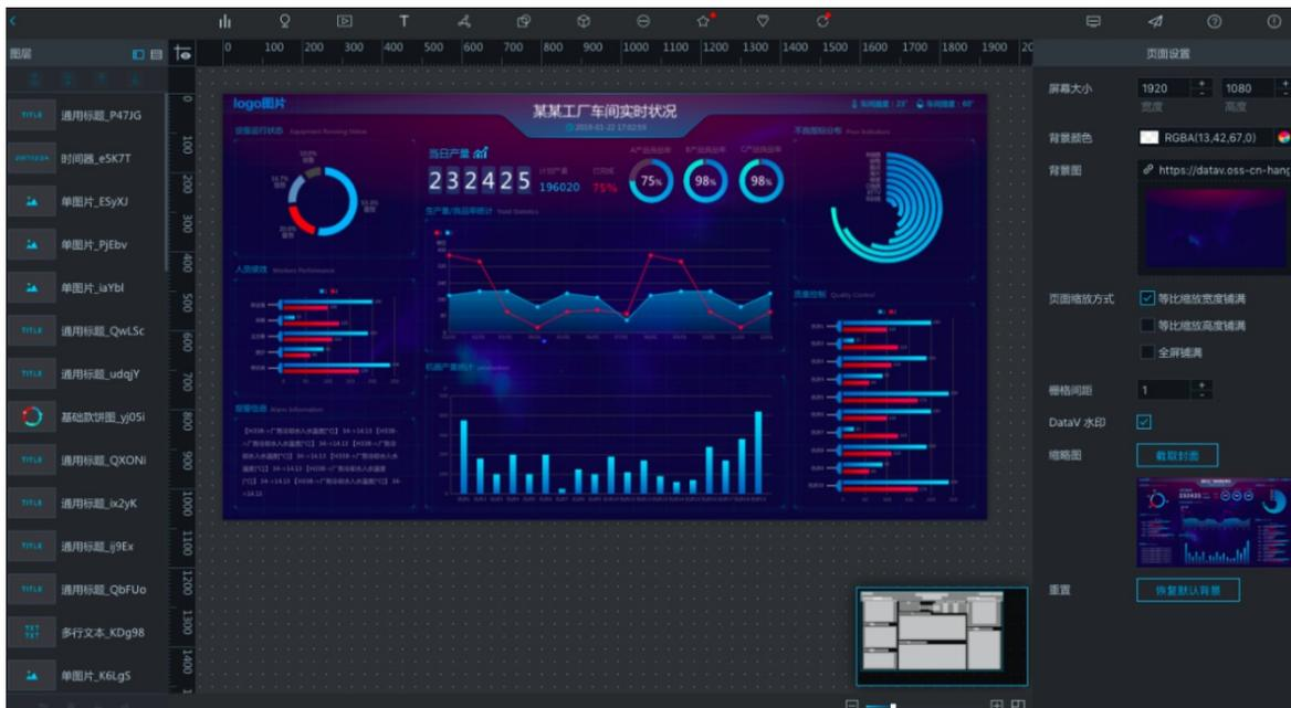
Widgets in the template contain static data. This example describes how to call the API to query the growth trend of the transaction amount and present the query results in the Basic Line Chart widget.
