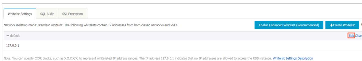
**6. In the Edit Whitelist dialog box that appears, enter the IP addresses or CIDR blocks used to access the instance, and then click OK. The following section describes the rules:**
