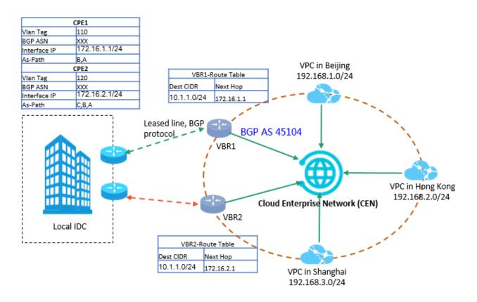
As shown in the following figure, the routing tables of VBR1 and VBR2 contain routing information and next hops learned from the BGP peers of VBR1 and VBR2. The VBRs, which are attached to the CEN, send the BGP routing information learned from the local data center to the CEN, including AS-Path properties.
