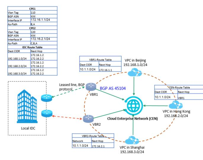
After attaching the VPC and VBR to CEN, the BGP route that the VBR learned are propagated to CEN. The CEN then synchronizes the routes to all attached networks based on the routing property.
