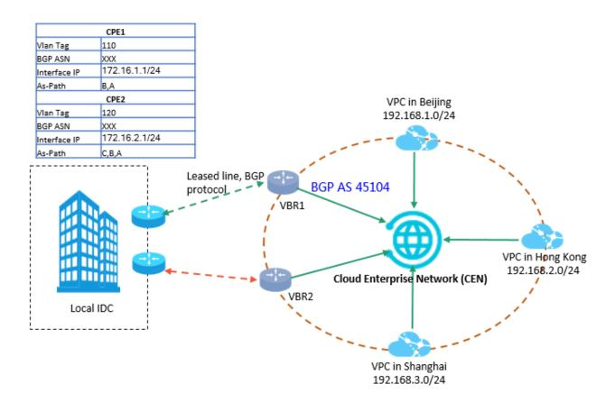
As shown in the preceding figure, the green link (CPE1) is the active link and the red one (CPE2) is the standby link. The BGP configurations of these two CPEs are as follows.
