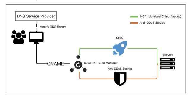
You can configure an Anti-DDoS Premium MCA instance for domain (7-layer) or port (4-layer).
