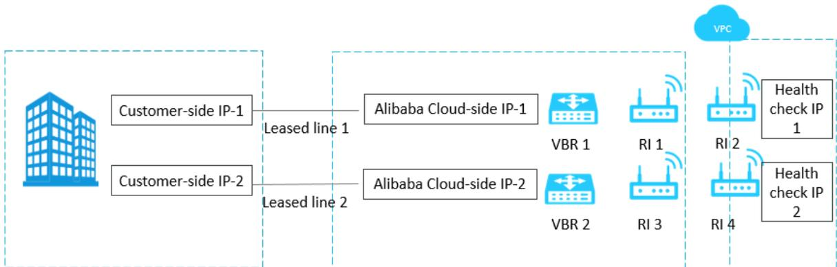
Alibaba Cloud sends a ping packet to the customer-side IP address of the local data center from each health check IP address every two seconds. If eight successive ping packets on one leased line fail to give response, the traffic is switched to the other leased line.
