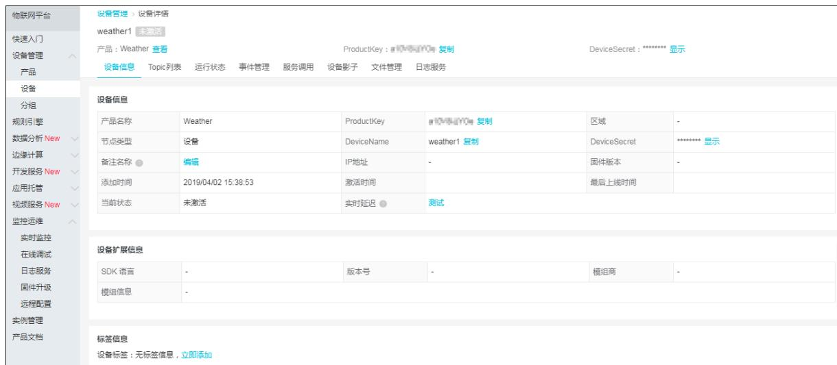
The screenshot shows the 'Device Management' section of the IoT Platform. On the left, there's a sidebar with various service categories. The main area displays a device named 'weather1' which is currently inactive ('未激活'). It provides details like ProductKey, DeviceName, IP address, and last online time. Below this, there are tabs for 'Device Extension Information' and 'Tag Information'. At the bottom, there's a note about adding tags.
