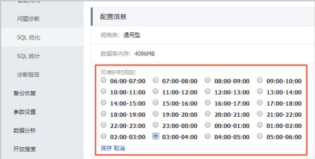
The screenshot shows the 'Configuration Information' (配置信息) section of the RDS console. It lists various parameters like '规格族: 通用型' and '数据库内存: 4096MB'. The '可维护时间段' (Maintenance Time) section is highlighted with a red box, showing a grid of radio buttons for 2-hour intervals. The '03:00-04:00' interval is selected. Below the grid are '保存' (Save) and '取消' (Cancel) buttons.
