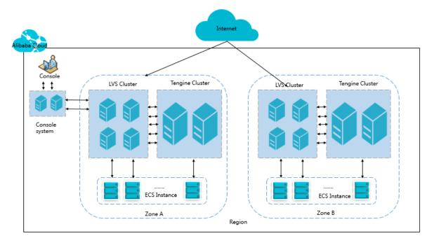
As shown in the following figure, Layer-4 Server Load Balancer in each region is actually run in a cluster of multiple LVS machines. The cluster deployment model strengthens the availability, stability, and scalability of the load balancing services in abnormal circumstances.
