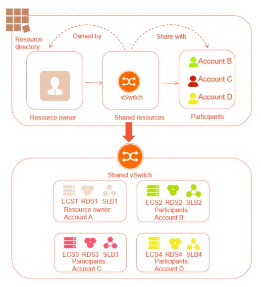
The following figure and descriptions provide details about how a VPC is shared.
