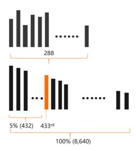
The average values of both inbound and outbound bandwidth are collected at intervals of 5 minutes. Whichever is greater between the average inbound and outbound bandwidth values is used as a data point. In this example, 288 data points are collected.
