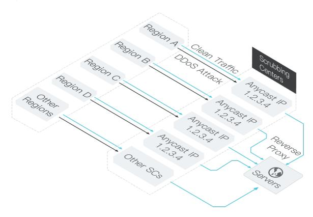
Traffic that reaches the anycast IP address can be routed to multiple data centers. When access traffic arrives at the anycast IP address, the traffic is forwarded to different data centers based on configured traffic forwarding rules. In most cases, the access traffic is forwarded to the data center nearest to the traffic source.
