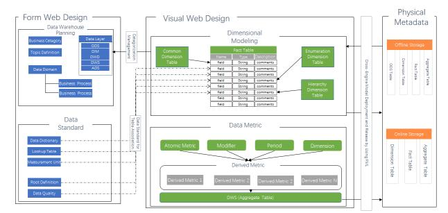
The following figure shows the architecture of each module of Data Modeling.
