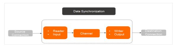
Before you synchronize data, you must connect the data sources to your resource group for Data Integration, as shown in the preceding figure. DataWorks allows you to use exclusive or custom resource groups for Data Integration to synchronize data. You can select a resource group type based on your business scenario. For more information about network connectivity solutions that can be used, see Select a network connectivity solution.
