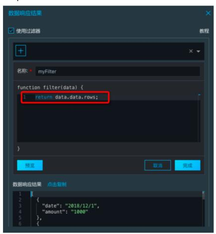
After you add a data filter, DataV can match data based on the specified fields.
