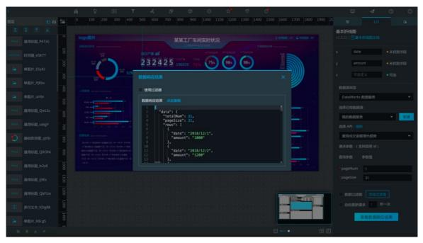
The preceding figure shows that the x and y fields match no data. This is because DataV has requirements for the data format and cannot identify fields with a deep structure. You need to add a data filter to filter out unnecessary fields.
